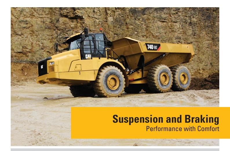
All three axles have oscillating A-frames with lateral tie rods, controlling sideways movement of the axle and providing stability. The suspension system allows the operator to travel at speed over rough terrain and softens impact loads on structures and components.
