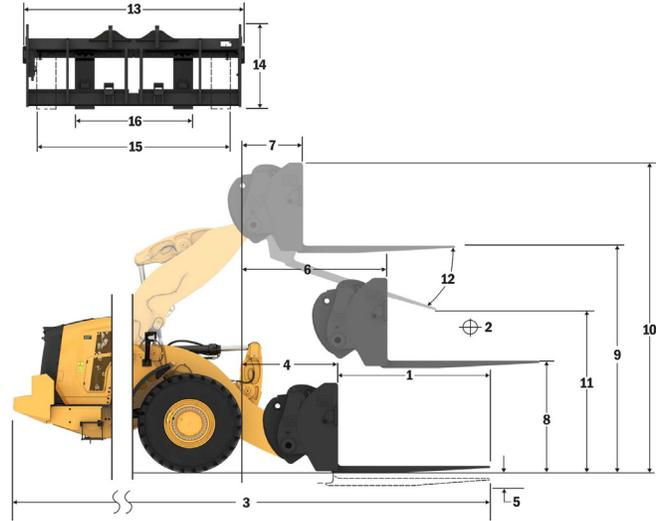
NOTE: Static tipping loads and operating weight are based on the following loader configuration: Bridgestone VJT L3 Tires, Air Conditioning, Ride Control, Powertrain Guard, Full Fluids, Fuel Tank, Coolant, Lubricants, and Operator.
