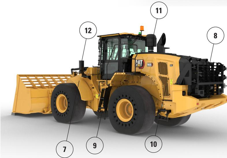
13. Lower front frame guard protects vital drivetrain components and keeps trash from getting in the front frame compartment
