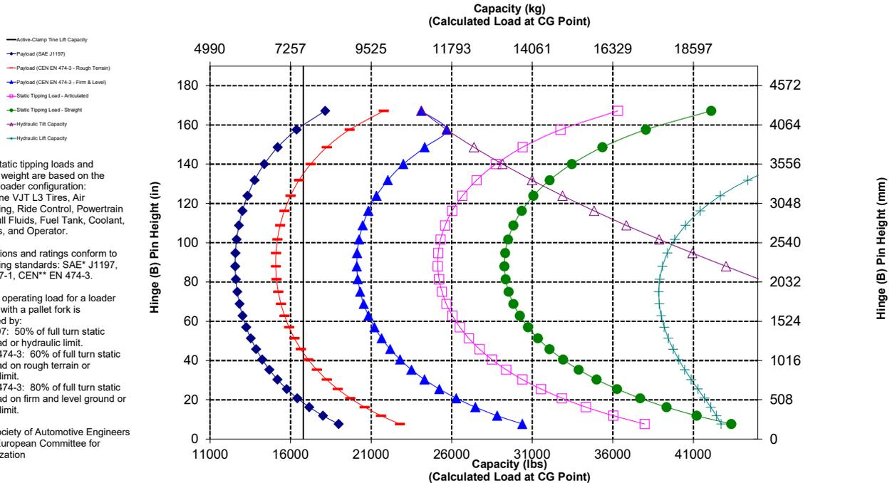
NOTE: Static tipping loads and operating weight are based on the following loader configuration: Bridgestone VJT L3 Tires, Air Conditioning, Ride Control, Powertrain Guard, Full Fluids, Fuel Tank, Coolant, Lubricants, and Operator.
