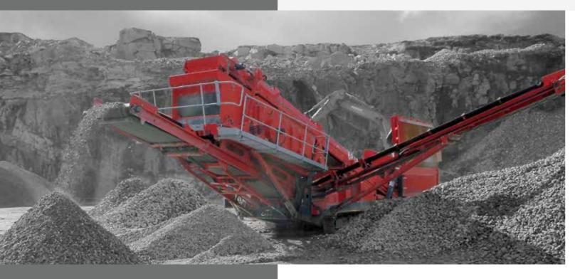
The Finlay® 684 inclined screen is a compact easily transportable machine that offers operators rapid set up and tear down times.
