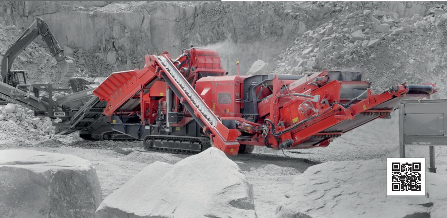
The Finlay® C-1540RS mobile cone crusher provides the versatility of a crushing and screening plant on one machine. Based on the Finlay C-1540 this machine features an innovative on board recirculating system and detachable sizing screen.
