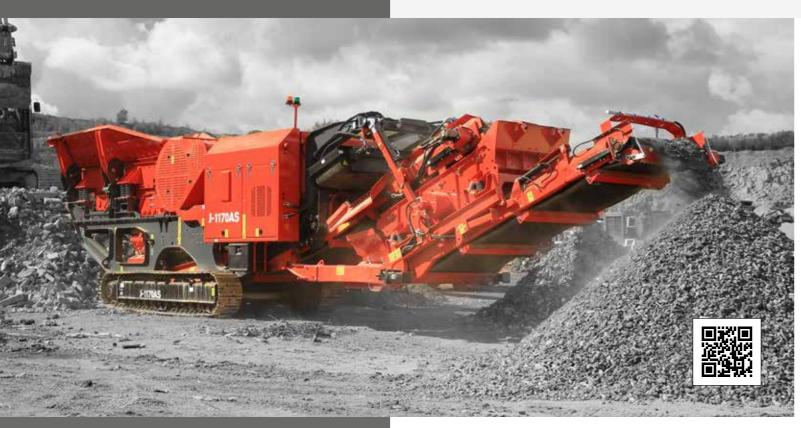
The Finlay® J-1170AS mobile jaw crushing plant provides the flexibility of a crushing and screening plant on one machine. This aggressive machine features a detachable on-board sizing screen.
