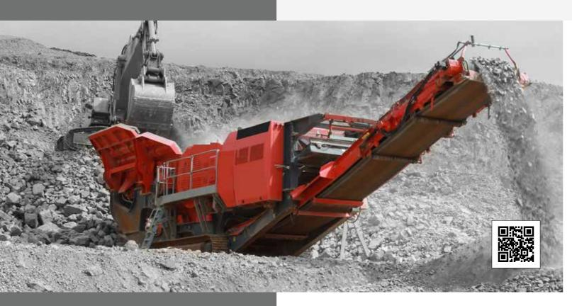
The Finlay® J-1480 incorporates the Terex Jaques JW55 single toggle jaw crusher which boasts a throughput capacity up to 750mtph depending on application and material.
